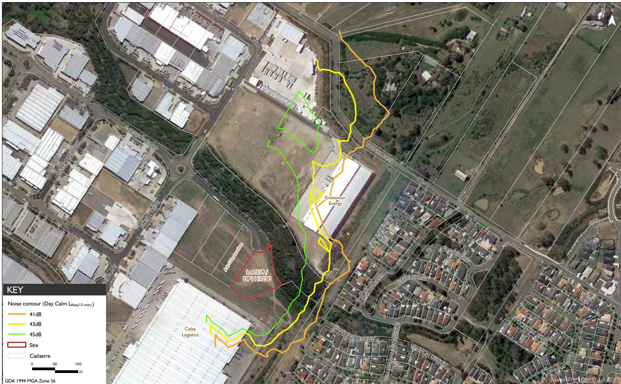
Predicted operational noise contours – Day Calm L_{Aeq}(15\text{-min})
